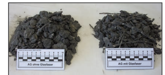
Asphalt granulate without glass fibres (left) and with glass fibres (right)
