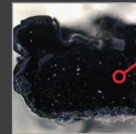
Filaments completely coated with an elastomeric polymer
