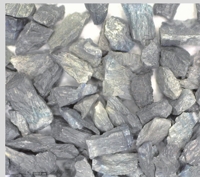
Macrostructure of mNZP® grains
